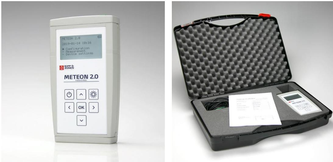
However, METEON 2.0 has a unique comparison mode that does most of the work for you. It sums the total irradiance during the logging period from each pyranometer and a report is generated in the logger that shows the difference between these two totals as a percentage. It cannot screen the data for outliers, so make sure that nothing affects the readings during the measurement period; such as shadows from site structures.
